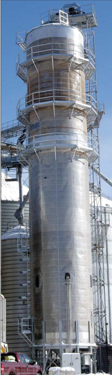
*New 4,700-bph Zimmerman tower dryer installed at Rock Springs, one of three Zimmerman dryers installed at cooperative locations in 2007.*
