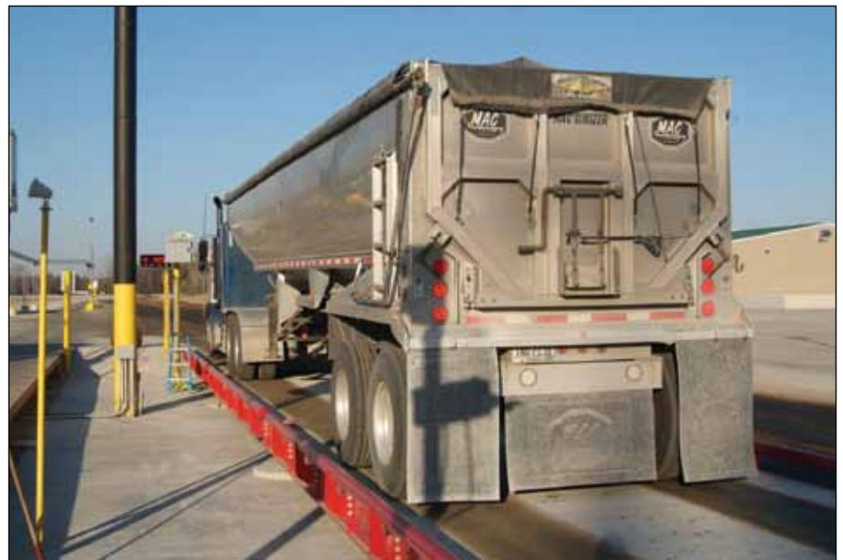
*Outbound truck is weighed on a new Rice Lake platform scale, while driver takes his scale ticket from a printer that is part of a CompuWeigh SmartTruck scale management system.*
