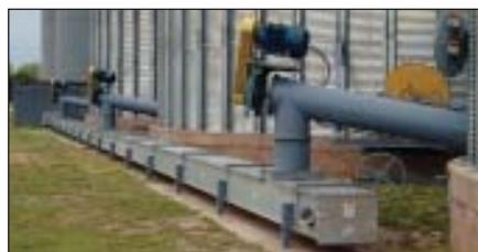
*Reclaim augers are used to empty the new steel tanks and deposit grain onto an above-ground InterSystems drag conveyor for return to an existing leg.*
