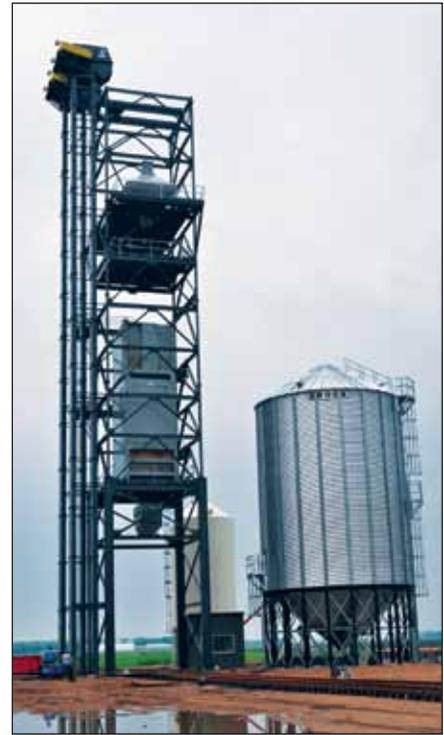
*Intersystems screener and bulk weigh scale are housed in a separate Warrior support tower directly over the loop track and are fed from a below-ground Schlagel enclosed belt conveyor and jump leg.*
