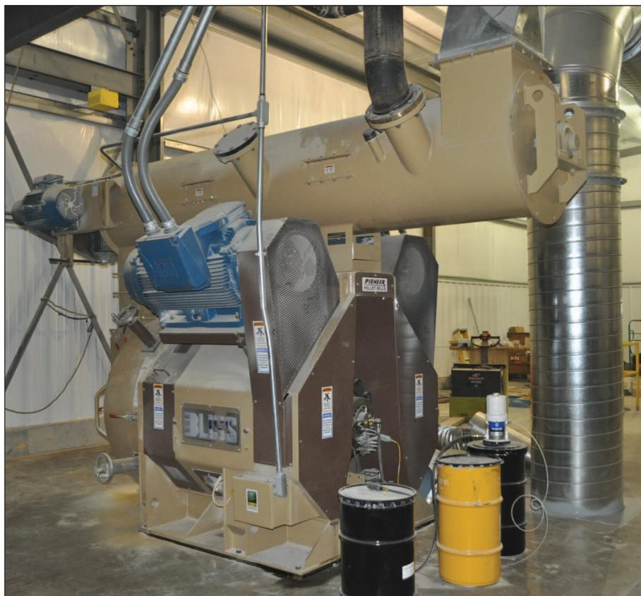
*Bliss 45-tph pellet mill is topped by a conditioner that allows up to 51 seconds retention time for incoming mash feed.*
